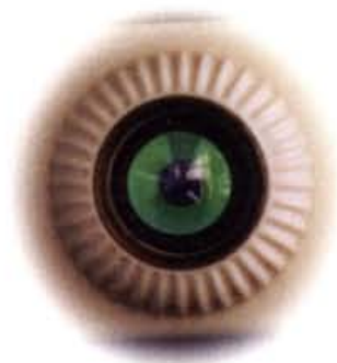
● Fig. 4: Believe it or not - there IS a volume control hidden around the 'Magic Eye' recording indicator! It fooled G4JCP and G3XFD. In fact Phil G4JCP even had to check on the circuit diagram to see if there was a volume control fitted! (see text).
