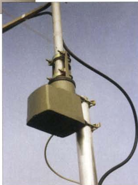
Fig. 2: The antenna rotator fitted onto Neill's Tonna 13-element antenna.
