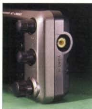
Fig. 7: The "VIDEO IN" port on the right-hand side of the IC-2800's head unit.
