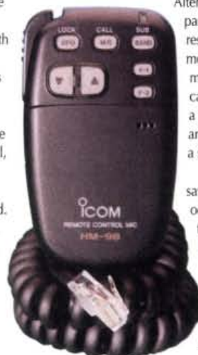
Fig. 2: The HM-98 microphone as supplied with the review IC-2100. It plugs into the front of the '2100. (Also see Fig. 1, far left).
