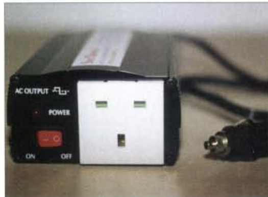
Fig. 4: The SkyTronic inverter end panel. Here you can see where the rotator plugs in and you can also see the ON/OFF switch.
