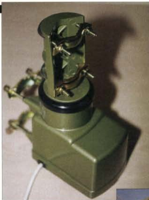
Fig. 1: The Altai HT127 antenna rotator which attaches to your mast and will fit onto a pole of up to 44mm diameter (though Neill managed to fit it on his 50mm mast) - it will also fit a stub mast up to 44mm (though this is the maximum).
