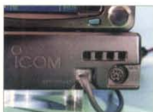
Fig. 5: The '2800 also comes with a supplied separation cable and a mini DIN socket for DATA applications (such as connecting a TNC).
